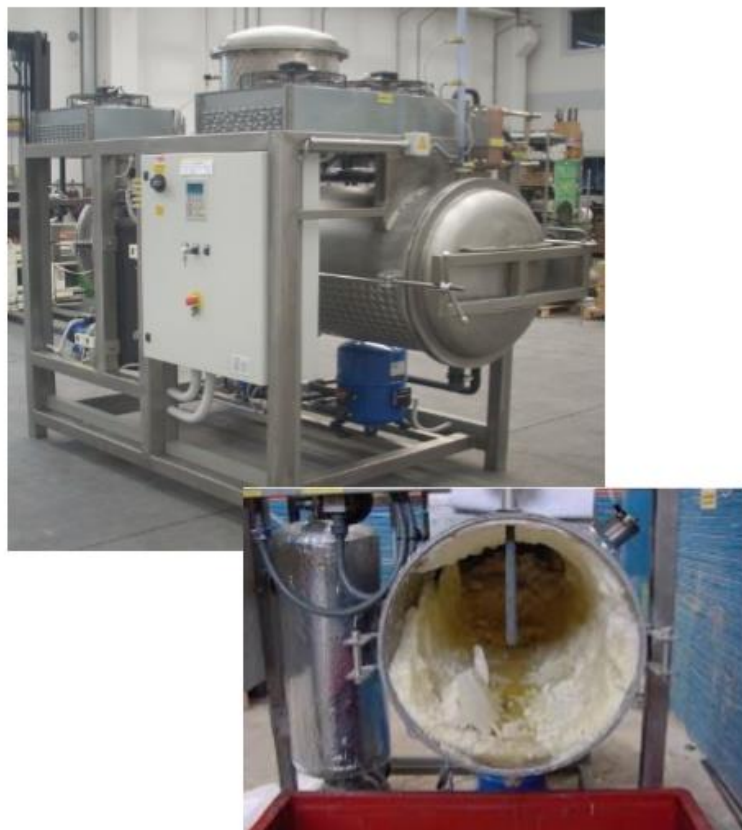
Figure 6.3 Brine Treatment System
